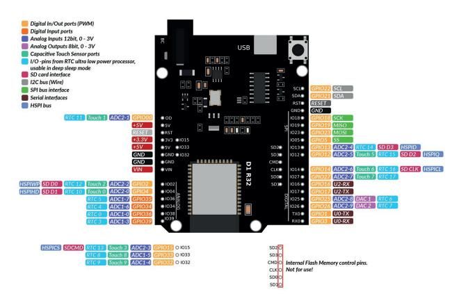
D1 R32 has digital input/output pins (GPIO pins - General Purpose Input/Output pins). These digital input/outputs operate at 3.3V.
